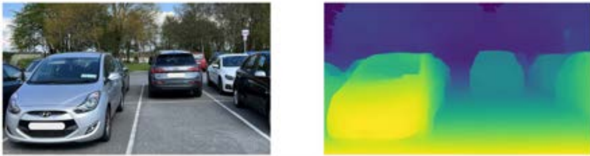
Figure 1: Left is original image and right is estimate depth with yellow being closest and black being furthest
